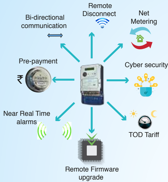
Figure 1: Smart Metering Components
